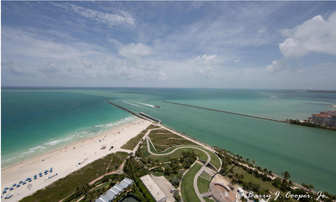
Figure 1. A turbidity plume can be observed to be leaving Biscayne Bay through Government Cut at PortMiami during dredging. Currents transported the sediment over the reef habitat offshore, even though dredging was occurring in Biscayne Bay and not offshore at this time. June 12, 2015.
